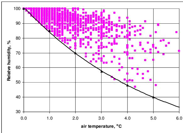
Fig. 1. The critical curve after eq.1 separating wet and dry snow events and the determined wet snow cases for station Bremerhaven
